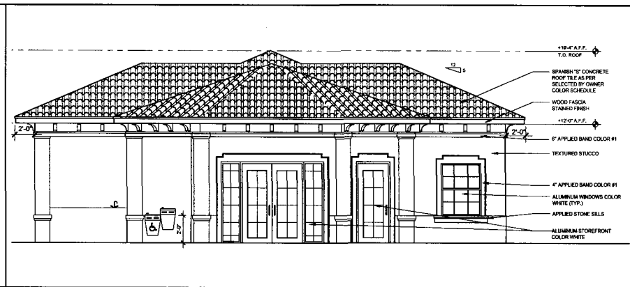
2 EAST ELEVATION SCALE: 1/4" = 1'-0"
