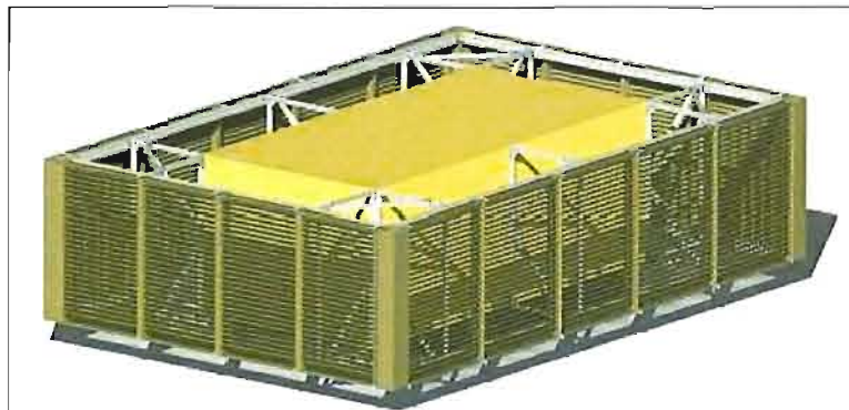
2 COOLING TOWER EQUIPMENT SCREENS SCALE: NTS
