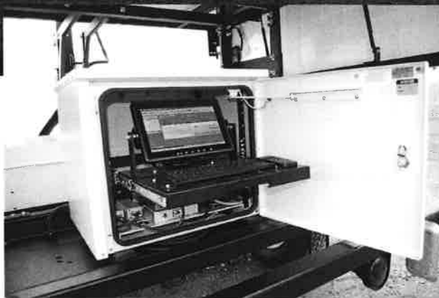
Control center in 9U NEMA housing
