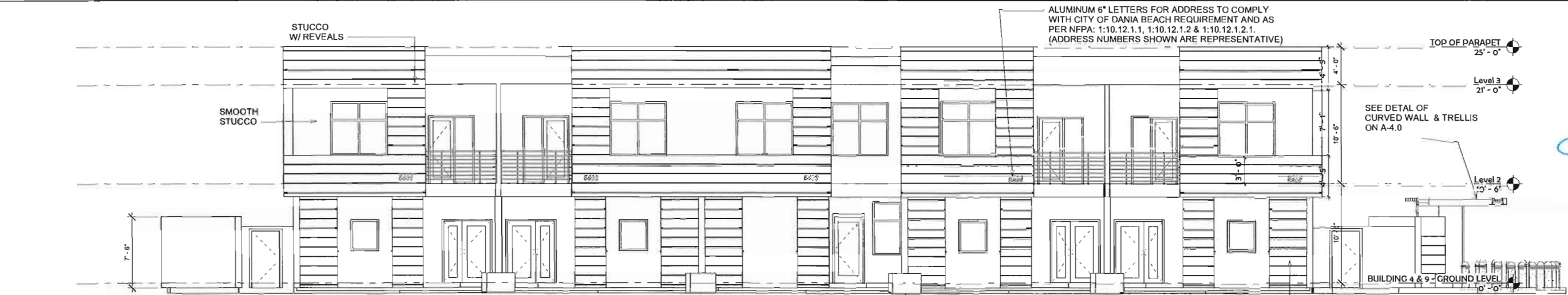
1 BUILDING 4 & 9 - FRONT ELEVATION 3/16" = 1'-0"
