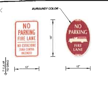
NO PARKING FIRE LANE SIGN SCALE: NTS
